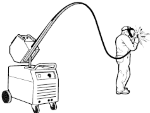
Figure 13. A load-reducing counter-balanced arm reduces the weight of the hoses through-out the working area.
