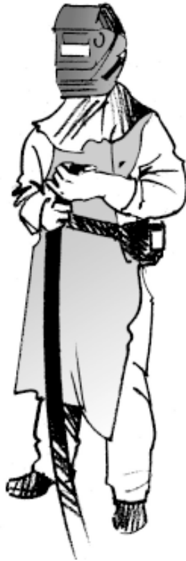
Fig. 6. Protection from UV, IR and visible light radiation is clothing with a leather apron and gloves and a welding helmet.
