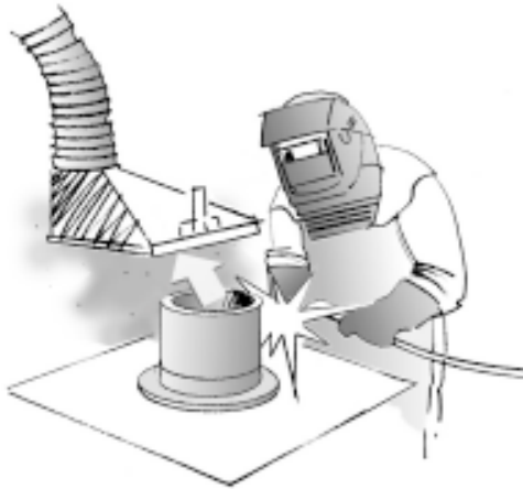
Fig. 8.Extraction and air treatment improve the air in the workplace and reduce the risk of injury to the people working there.
